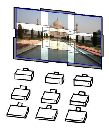
Setup for multiple projectors to create high resolution display
